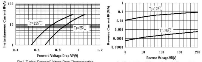
Fig.1-Typical Forward Voltage Drop Characteristics
