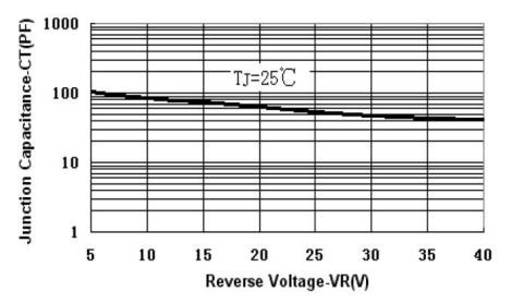
Fig.3-Typical Junction Capacitance Vs.Reverse Voltage
